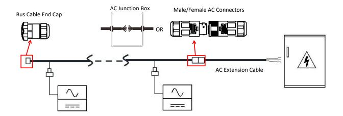
When AC extension cable is needed, users could connect the AC bus cable and AC extension cable in a junction box or use a pair of male/female AC connectors that APsystems provides as optional accessory.
